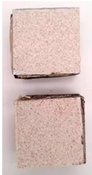
Fig. 3 Example of type of failure after test on reference 2108071-02
