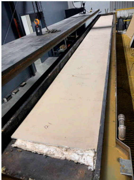
Photo No. 4 Post-Test Unexposed Side in Tunnel
