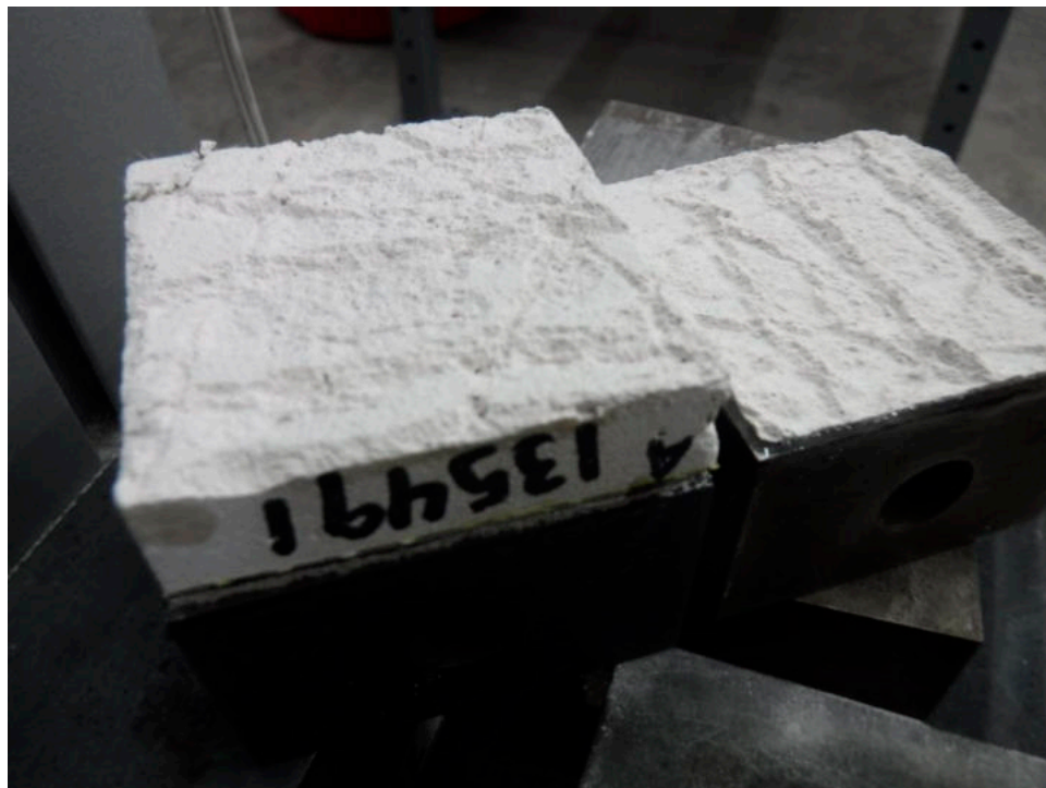
Photo No. 2 Core Failure Example, Specimen Number 135491
