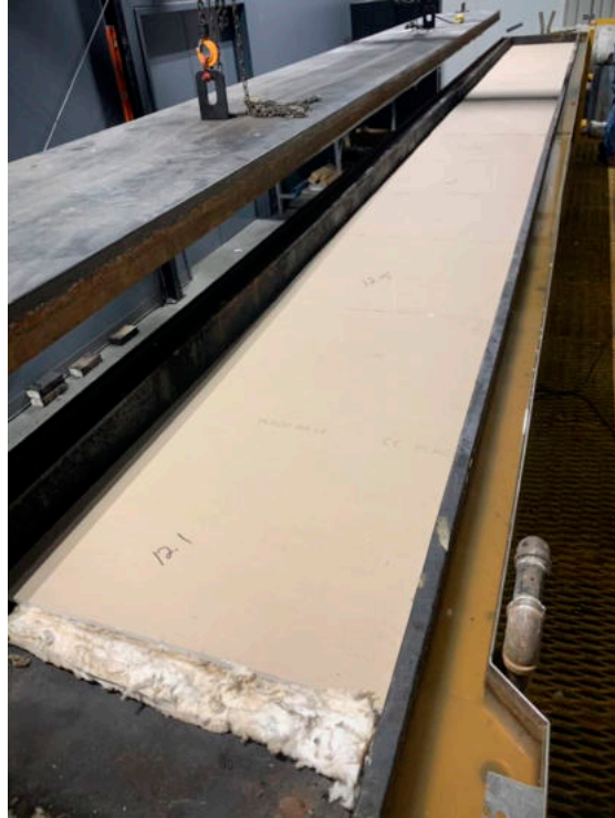
Photo No. 3 Pre-Test Unexposed Side in Tunnel
